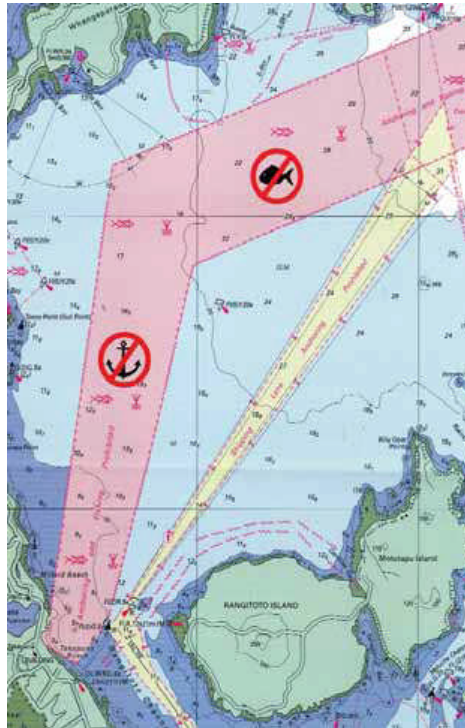
Figure 7.7: Cable protection zone New Zealand
