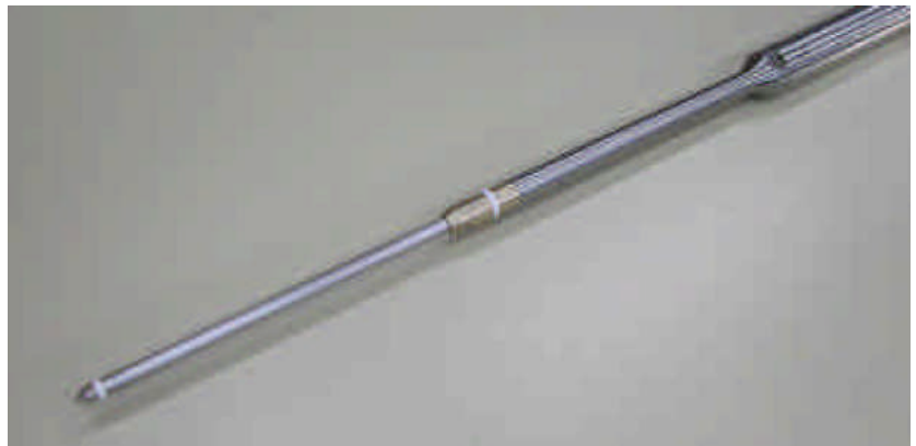
Figure C.12: Pore Pressure Probe
