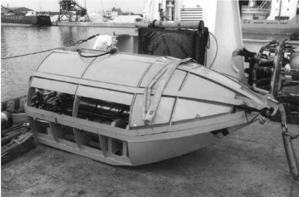
Figure 6.6: GAMBAS – Tow Sled for Seismic Refraction [Ref. 6.14]
