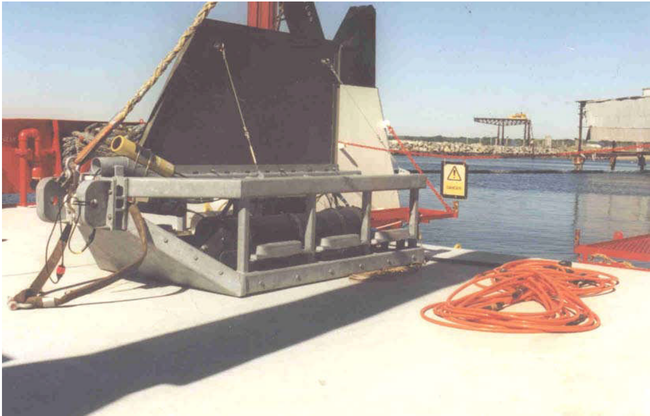
Figure 6.5: Typical Burial Assessment Survey Sled [Ref. 6.9]
