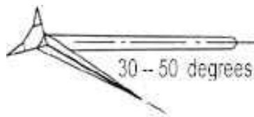
Figure 7.4 Fluke Angle of Typical Ship Anchor
