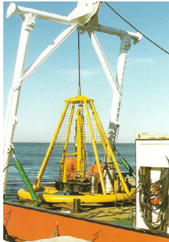
Figure C.10: The SEAROBIN is one of the widely used CPT units for determining the soil for the route assessment.
