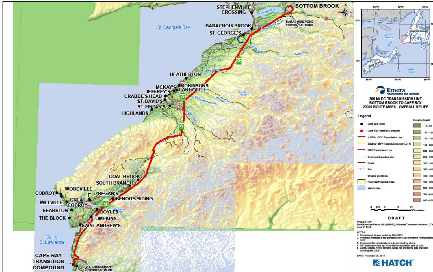
Figure 3-1: HVdc Transmission Line Route in Newfoundland
