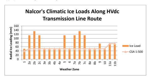
Figure 9: Climatic Ice Loads along the HVdc Transmission Line Route compared to the CSA Standard 1:500-year return period limit
