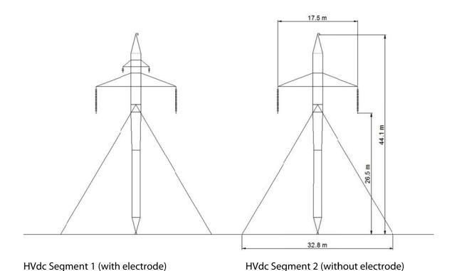
Figure 8: Typical HVdc Transmission Guyed Tangent Structures which comprise approximately 85% of the towers in the Labrador-Island HVdc transmission line
