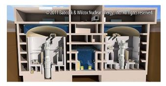
Conceptual drawing of an underground containment structure housing two B&W mPower reactor modules. Drawing from B&W Nuclear Energy, Inc.
