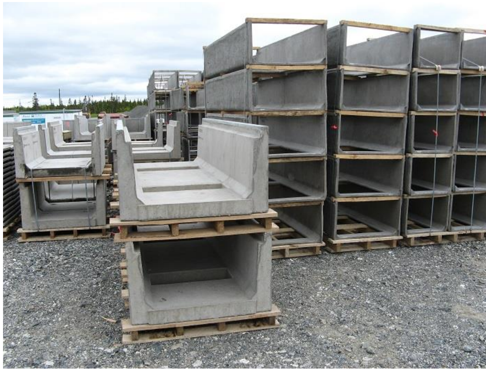
Photo 25 - Precast concrete sections for cable ducts.
