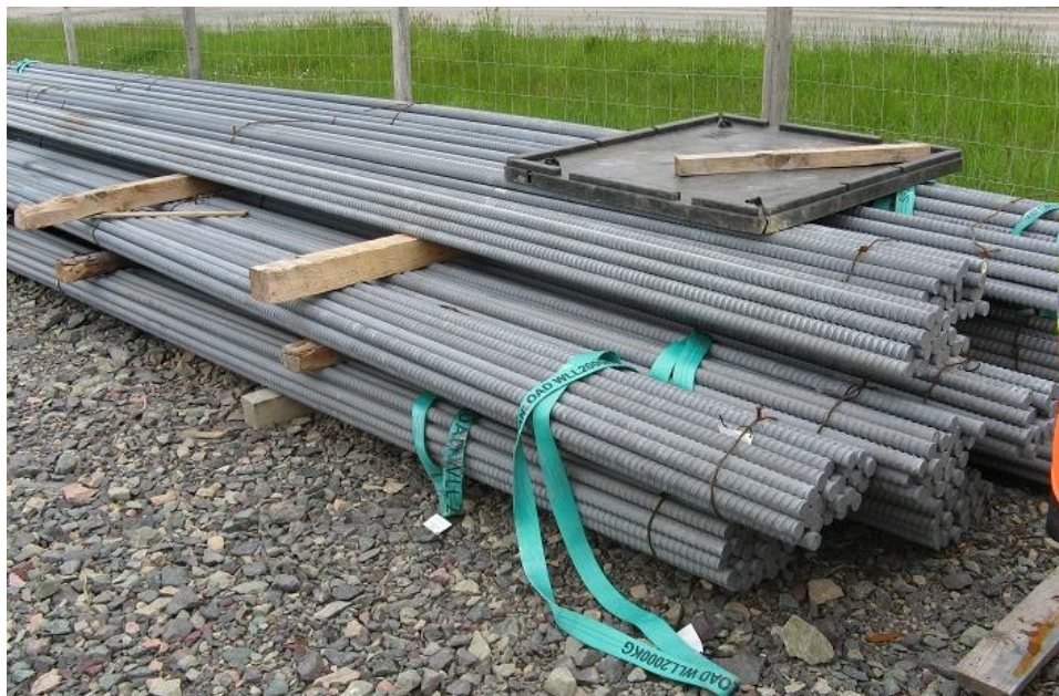
Photo 9 - Threadbar anchors for tower footings.
