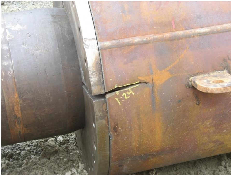
Photo 5 - Crack in casing hammer resulting from driving casing against high resistance.
