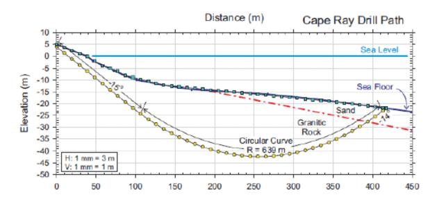
Figure 2: Cape Ray NL HDD Conceptual Design
