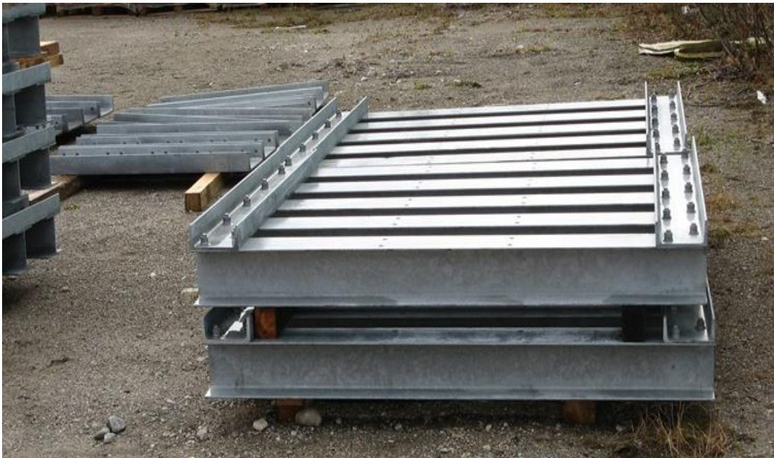
Photo 16: Abengoa materials storage yard – sample of foundation grillage, assembled by trainees.
