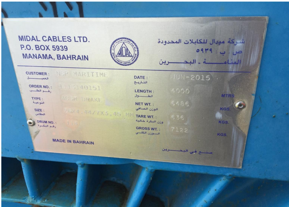
Photo 14: Abengoa materials storage yard – ACSR (Aluimnum Clad Steel Reinforced) Drake / HVAC Conductor.
