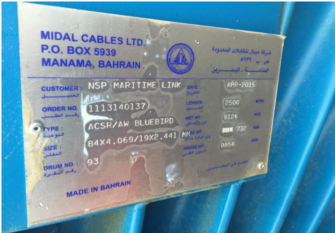
Photo 13: Abengoa materials storage yard – ACSR (Aluimnum Clad Steel Reinforced) Bluebird / HVDC Conductor.
