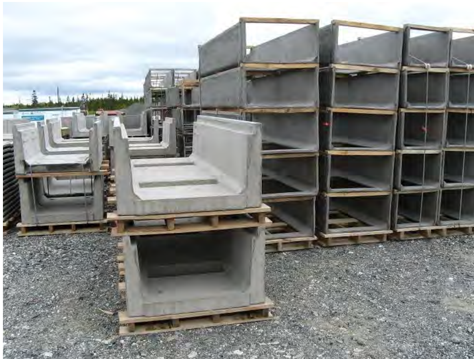
Photo 25 - Precast concrete sections for cable ducts.
