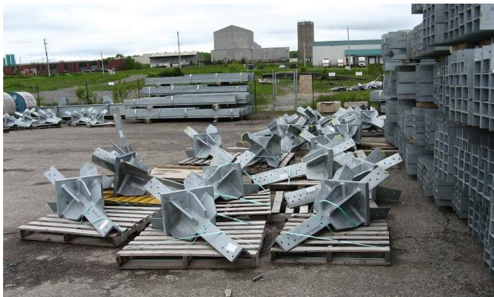
Photo 11 - Grillage footing components.
