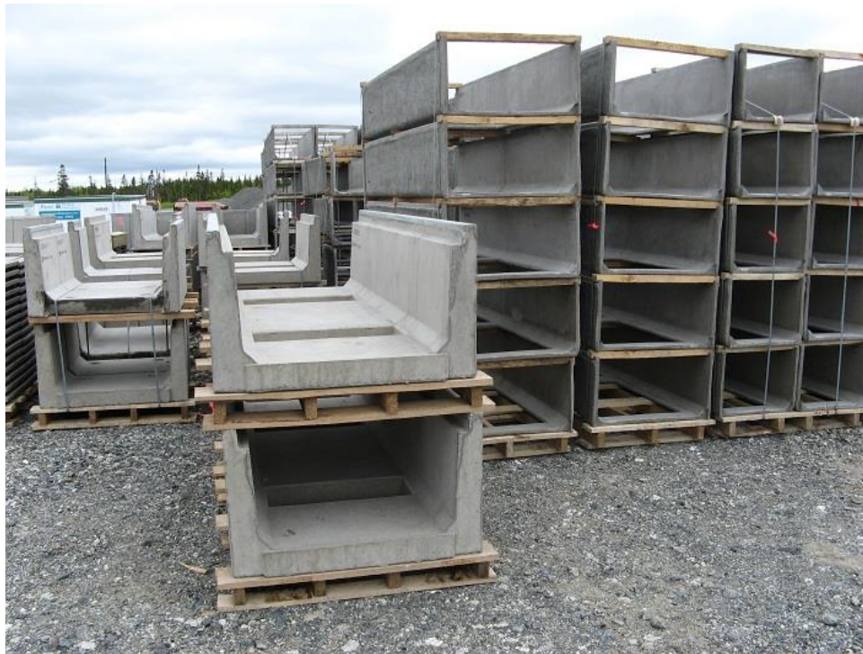
Photo 25 - Precast concrete sections for cable ducts.
