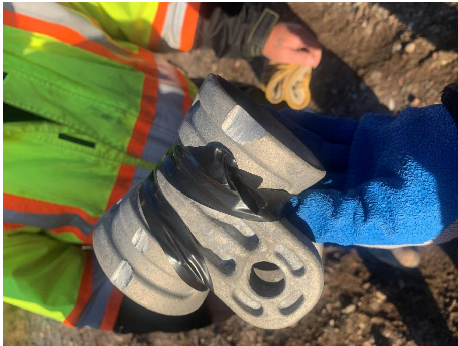
Photo 3: Damaged shield wire / OPGW clamp
