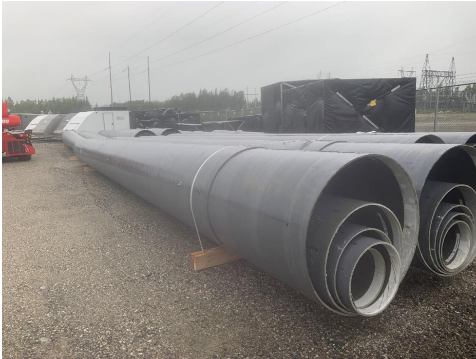
Photo 6: Storage facility - Emergency spare FRP (Fiber reinforced) poles
