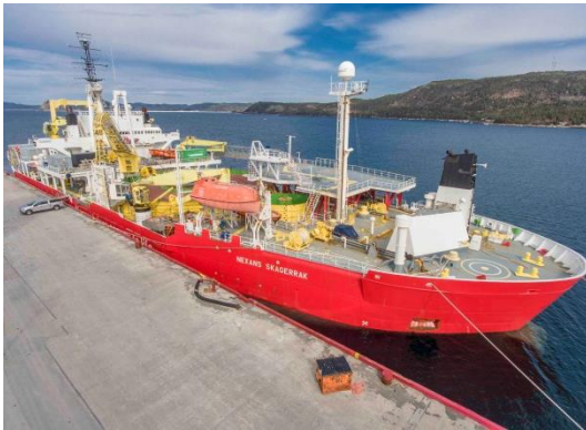
The Skagerrak was built in 1976 and refurbished in 2010 to enhance cable handling capability.
