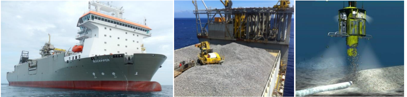
The Rockpiper will be the base of operations for protective rock berming activities.
