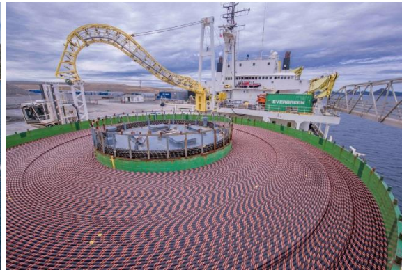
The cable turntable on the Skagerrak holds a 170 km submarine cable for the Maritime Link.
