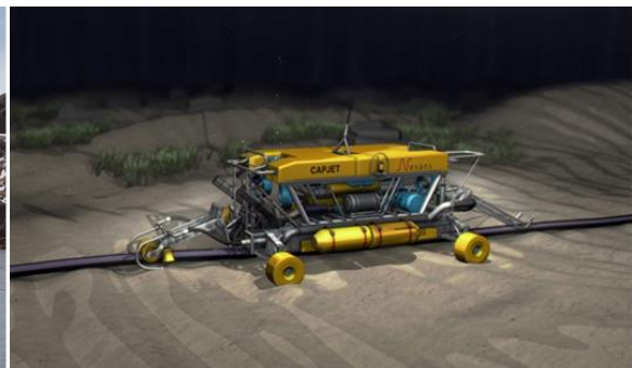
Nexans ROV, the Capjet, will be used to perform cable trenching for the Maritime Link's submarine cables.
