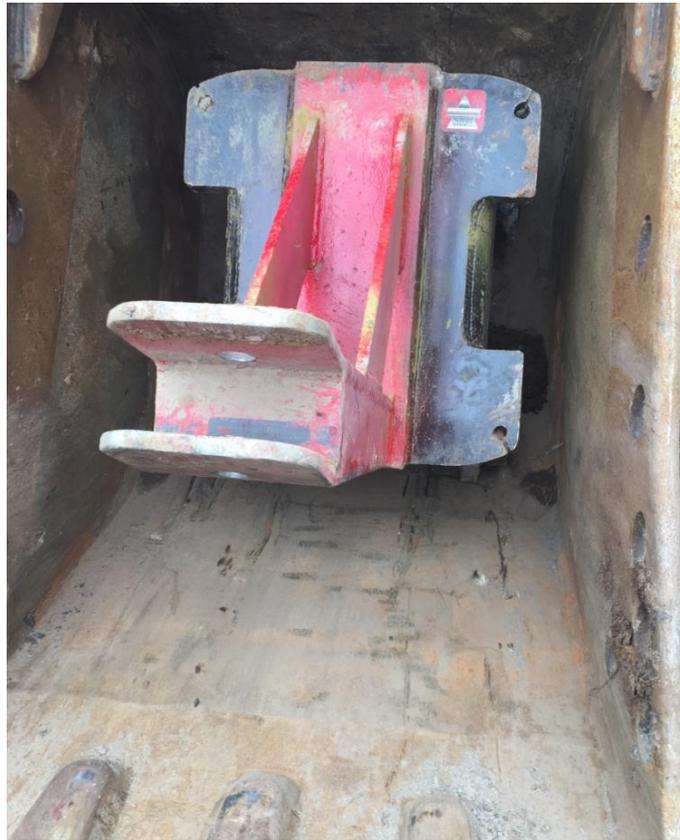
**Photo 10:** HVDC – This attachment was developed to hold one guy connection at the tower while working on the 4 anchors.
